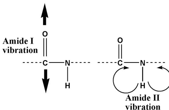
Figure 2. Amide I and Amide II band vibrations in the infrared spectrum of BSA protein
