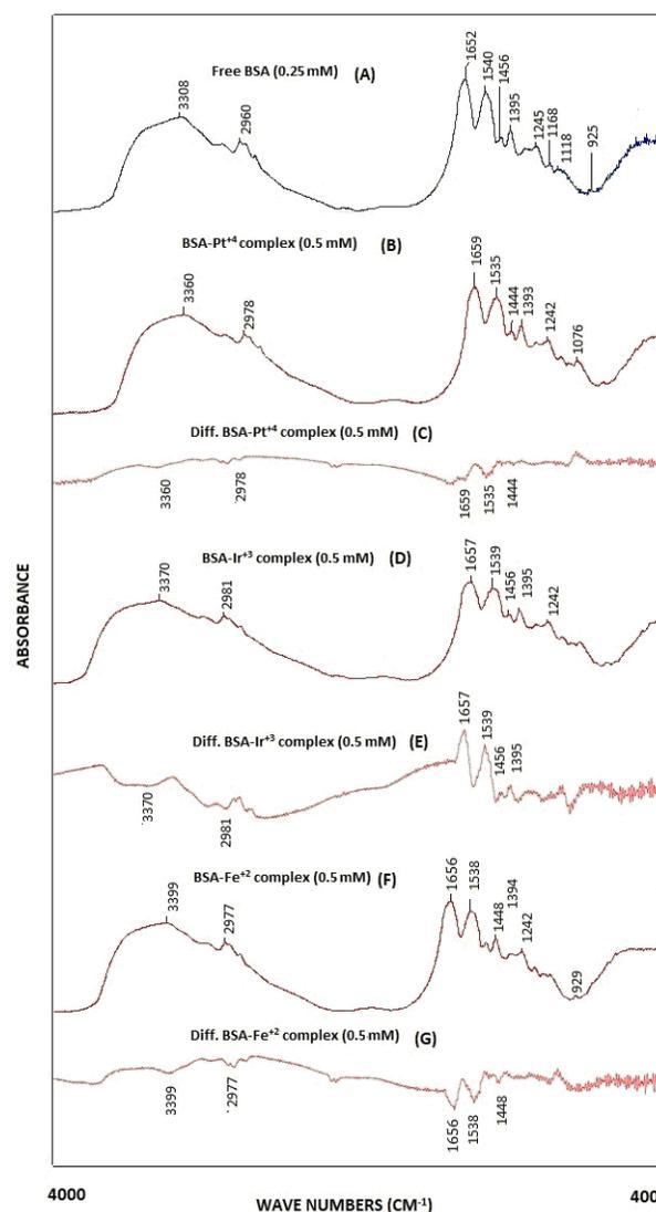
Figure 3. FT-IR spectra of (A) free BSA (0.25 mM) (B) Pt(IV)-BSA complex (0.5 mM) (C) Diff. Pt(IV)-BSA complex (0.5 mM) (D) Ir(III)-BSA complex (0.5 mM) (E) Diff. Ir(III)-BSA complex (0.5 mM) (F) Fe(II)-BSA complex (0.5 mM) (G) Diff. Fe(II)-BSA complex (0.5 mM)
