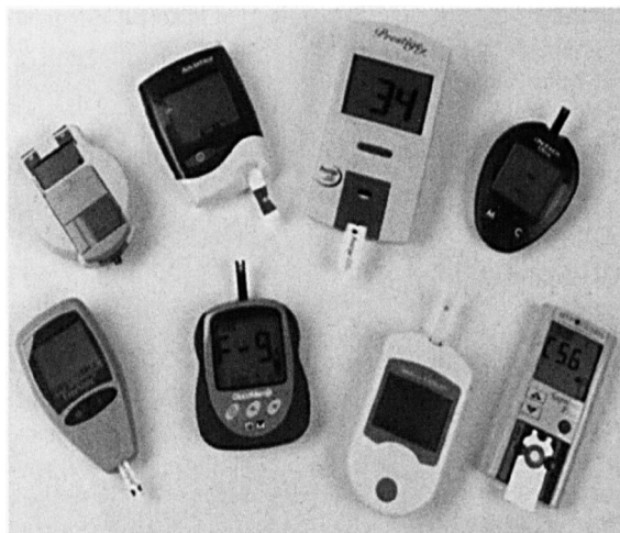
With the 21st century came a number of different electrochemical glucose meter systems, including the OneTouch Ultra (top right) from Johnson & Johnson. See this image in colour at www.bjbs-online.org
