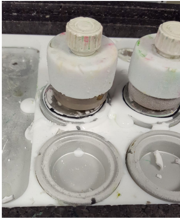
Figure 3. The freezing embedding chambers/wells of the PrestoCHILL Cryoembedding System. Note two wells are 25 mm in diameter and two are 35 mm in diameter.
