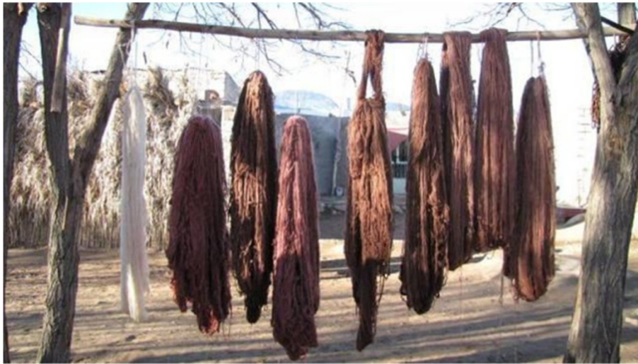
Figure 14 Cashmere yarn is dyed using natural dyes such as Henna, Rubbia and walnut husk. Dyed yarn is cooled, washed, rinsed and hanged to dry.
