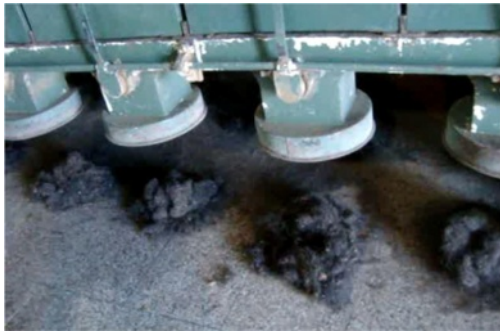
Figure 17 Guard hair and cashmere waste is discarded from the exit valves beneath the garneting machine. Mashad processing mill in Khorasan Razavi Province. October 2011
