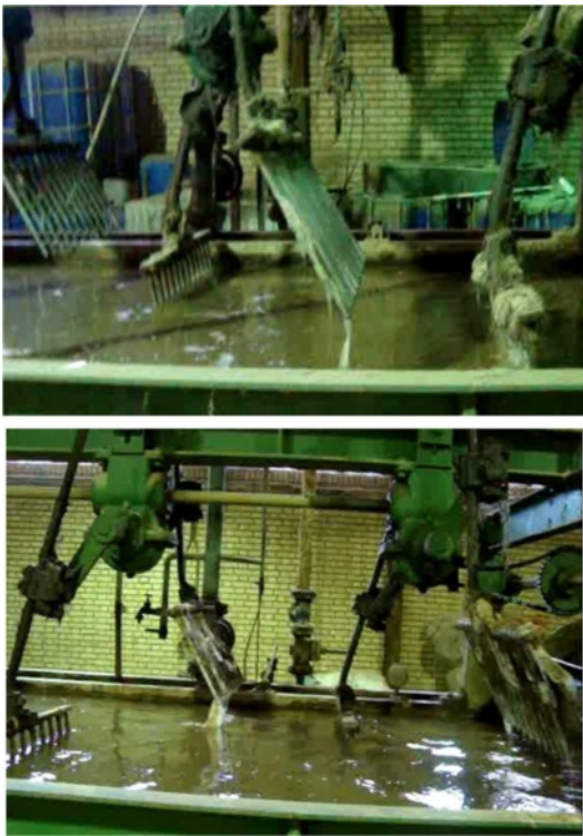
Figure 13 Cashmere scouring machine: first and second bowl propulsion and extraction by harrows. Sefit Pajan processing mill in Semnan Province. October 2011
