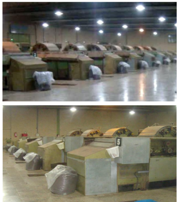
Figure 19 Cashmere dehairing machines. Mashad processing mill in Khorasan Razavi Province. October 2011
