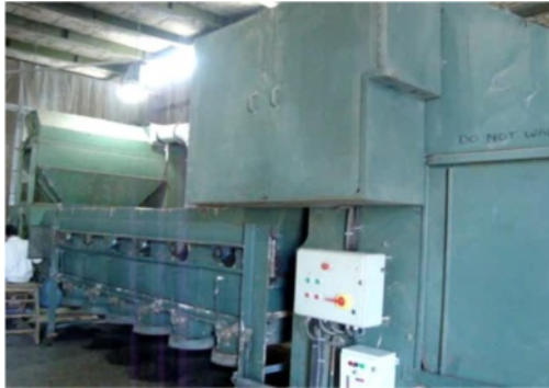
Figure 16 Garneting machine. Short cashmere fibre is manually fed into the machine. Mashad processing mill in Khorasan Province. October 2011
