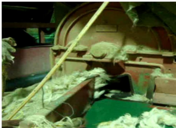
Figure 12 Double-cylinder cashmere opener. Sefit Pajan processing mill in Semnan Province. October 2011
