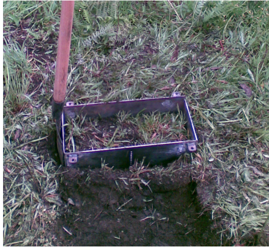
Figure 1. Soil sampling using steel boxes 20 x 40 x 15 cm to preserve soil structure.
