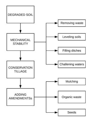
Figure 4. General restoration process of a quarry (own source).
